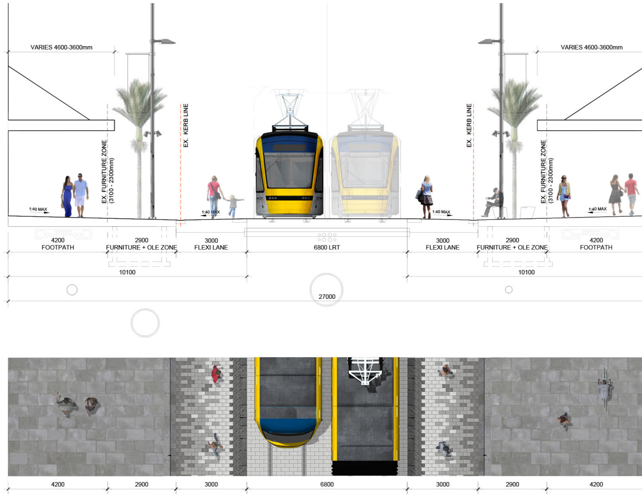
Figure 43 Partial plan and section of Queen Street between Wellesley Street and Customs Street looking north. Centrally located carriageway with through vehicular traffic removed. servicing provided at offpeak hours via 3000-3500mm
