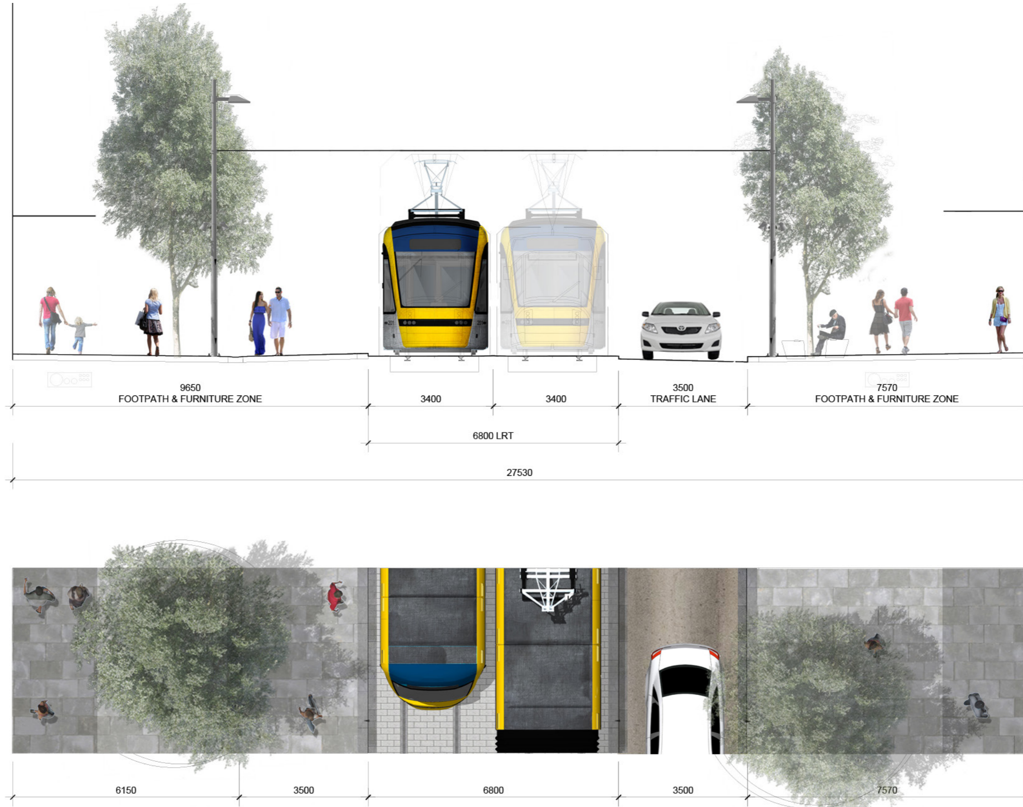
Figure 51 Cross section of Queen Street between Mayoral Drive (south) and Airedale Street (north) looking north towards Aotea Square. Centrally located LRV carriageway with adjacent south band traffic lane running between Wakefield Street and Mayoral Drive.
