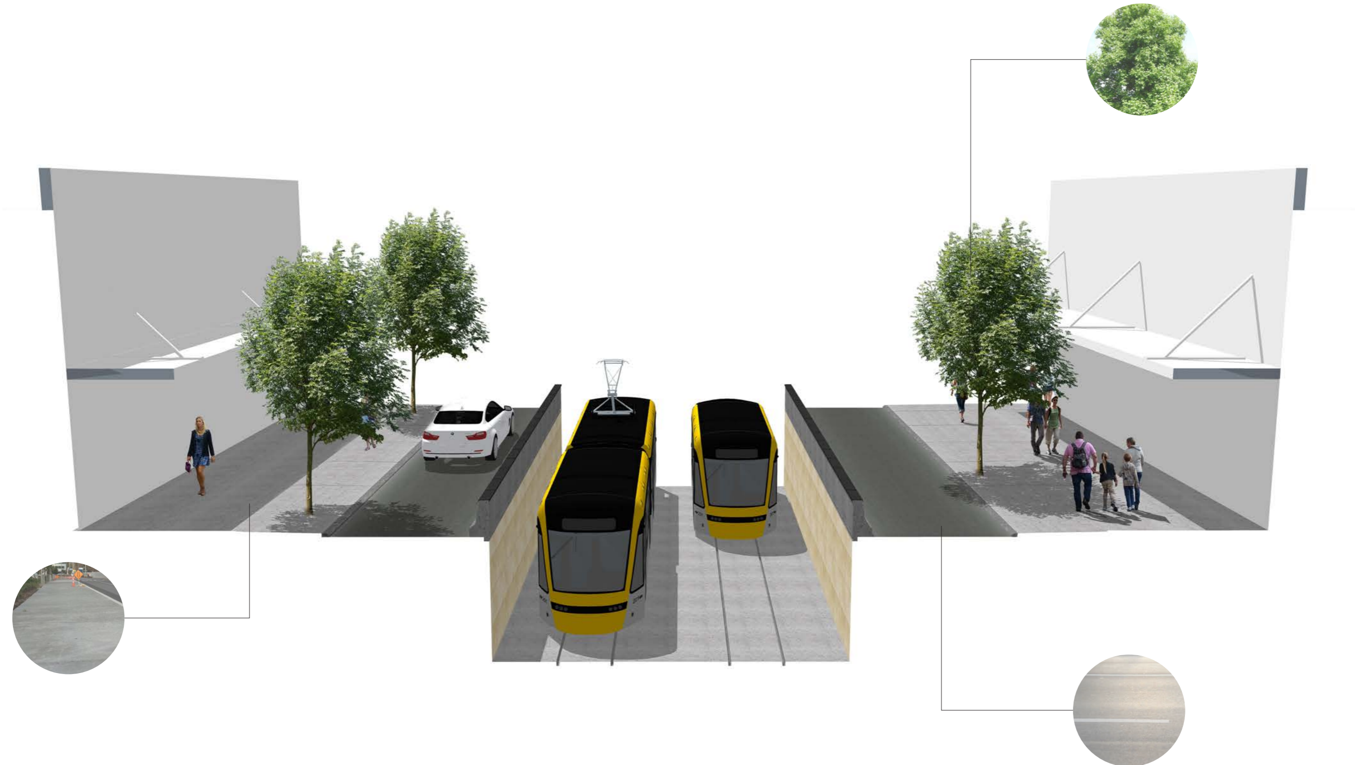
Figure 60 Sectional Perspective of existing Upper Queen Street portal with LRV carriageway underpass and indicative streetscape treatments. Existing significant (Liriodendron) street trees retained where possible or replaced with additional native trees in similar locations.
